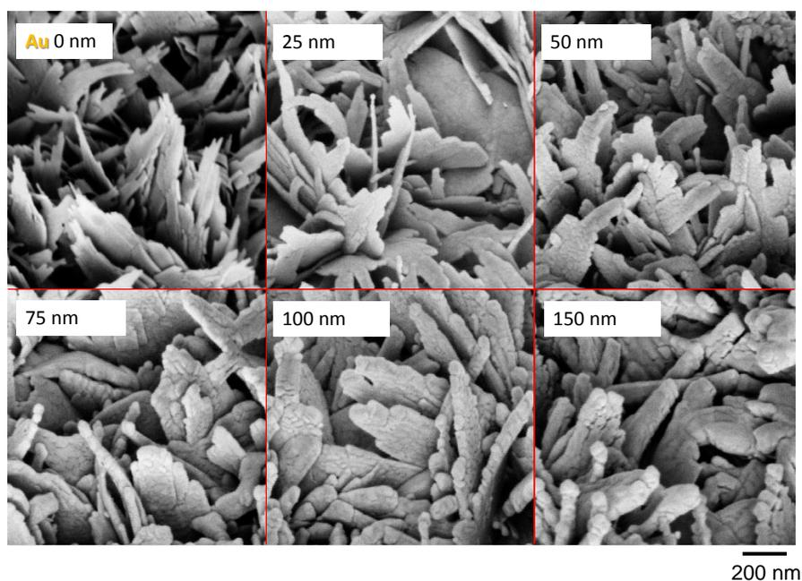
**Fig. 1** Conformal coating: SEM images of black CuO with different thicknesses of sputtered Au, viewed from a 45°-tilt angle. Magnification = 30,000×. The indicated thicknesses are taken from the flat reference surface.
