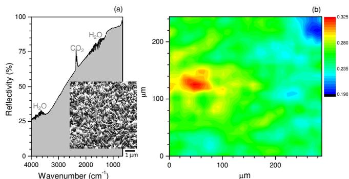
**Fig. 3** (a) Reflectivity of black CuO measured by FTIR; spectral regions with artefacts due to CO<sub>2</sub> and H<sub>2</sub>O absorption bands are labelled. Reflectivity was normalized to a Au mirror of  $R \equiv 1$ . Inset shows an SEM image of the sample. (b) FTIR map of reflectivity over an extended area measured with 6.25  $\mu\text{m}$  spatial resolution.
