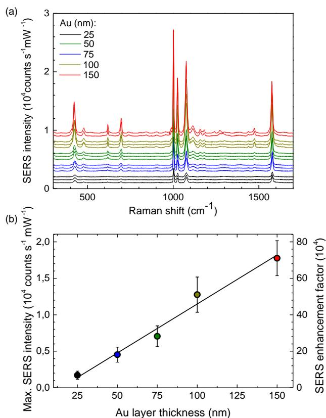
**Fig. 4** (a) SERS of thiophenol for different thicknesses of Au coating. Excitation wavelength was 785 nm and SERS intensity was normalised by the excitation power. (b) SERS intensity of the 1001  $\text{cm}^{-1}$  thiophenol peak as well as the estimated SERS enhancement factors plotted against Au thickness.
